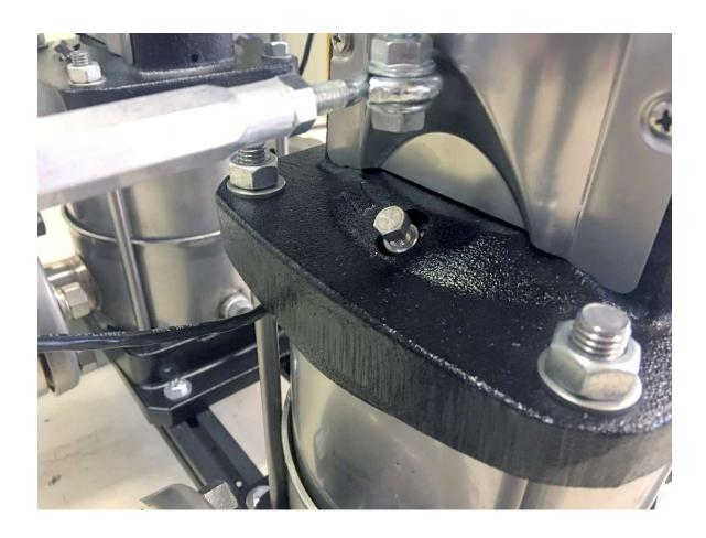
TURN THIS PLUG CCW UNTIL AIR IS RELEASED, IT DOES NOT NEED TO BE TOTALLY TURNED OUT. ONCE ALL AIR IS RELEASED THERE WILL BE ONLY WATER BEING RELEASED. TIGHTEN PLUG BACK UNTIL WATER STOPS LEAKING. DO NOT OVER TIGHTEN THIS PLUG.
