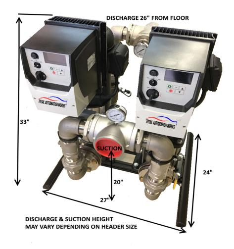
NOTE: DISCHARGE AND SUCTION HEADERS CAN BE REVERSED BY REMOVING THE HEADER AT THE UNION AND TURNING IT AROUND 180 DEGREES. THIS ALLOWS THE DISCHARGE TO FACE FORWARD AND THE SUCTION TO FACE BACK. **OPPOSITE FROM THE PICTURE ABOVE.**
